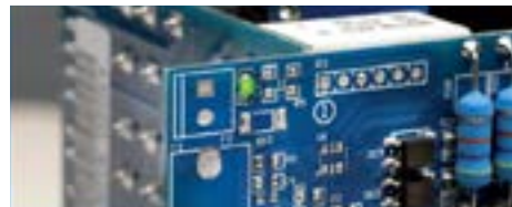
LED lights to indicate: Power supply ON (green), actuator working conditions (yellow) and fault (red).
