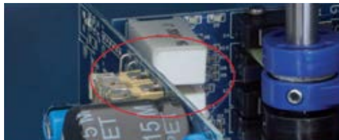
Heating resistor Managed by the control board to guarantee the right internal temperature
