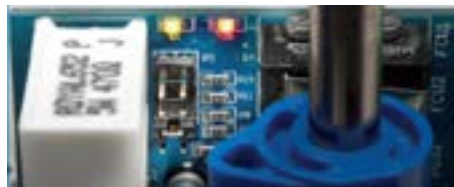
LED lights to indicate: Power supply ON (green), actuator working conditions (yellow) and fault (red).
