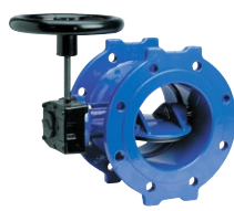
Series 756/100 Butterfly valve Double eccentric Double flanged Integral seat IP 67 gearbox DN150-2800 PN10/16 Ductile iron
