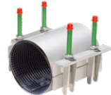
Series 748/02 Repair clamp Double band Stainless steel AISI 304 or AISI 316 NBR or EPDM rubber Options: • handgrip
