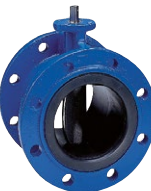
Series 75/21 Butterfly valve Centric with fixed liner Double flanged long DN50-1500 PN10/16 Ductile iron
