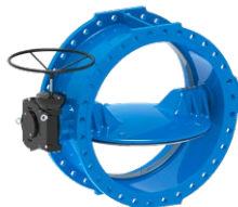
Series 756/106 Butterfly valve Double eccentric Double flanged Integral seat IP 68 gearbox DN150-2800 PN10/16 Ductile iron
