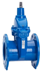
Series 06/35 Flanged gate valve with position indicator Face-to-face DIN F4 DN50-400 PN10/16 Ductile iron
