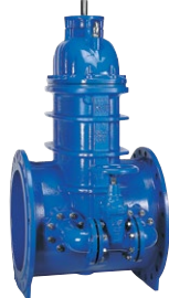
Series 55/30 Flanged gate valve DN450-500-600-800 Face-to-face DIN F5 PN10/16 Ductile iron Resilient seated Replaceable stem sealing
