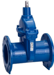
Series 02/60 Flanged gate valve Face-to-face DIN F5 DN40-500 PN10/16 Ductile iron
