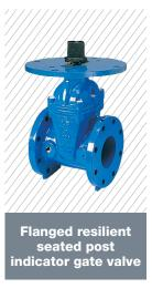
Body and bonnet in ductile iron. Stem in stainless steel Wedge in ductile iron vulcanized with AVK EPDM rubber. Fusion bonded epoxy coating acc. to GSK Operated by Post Indicator. UL/FM approved.
