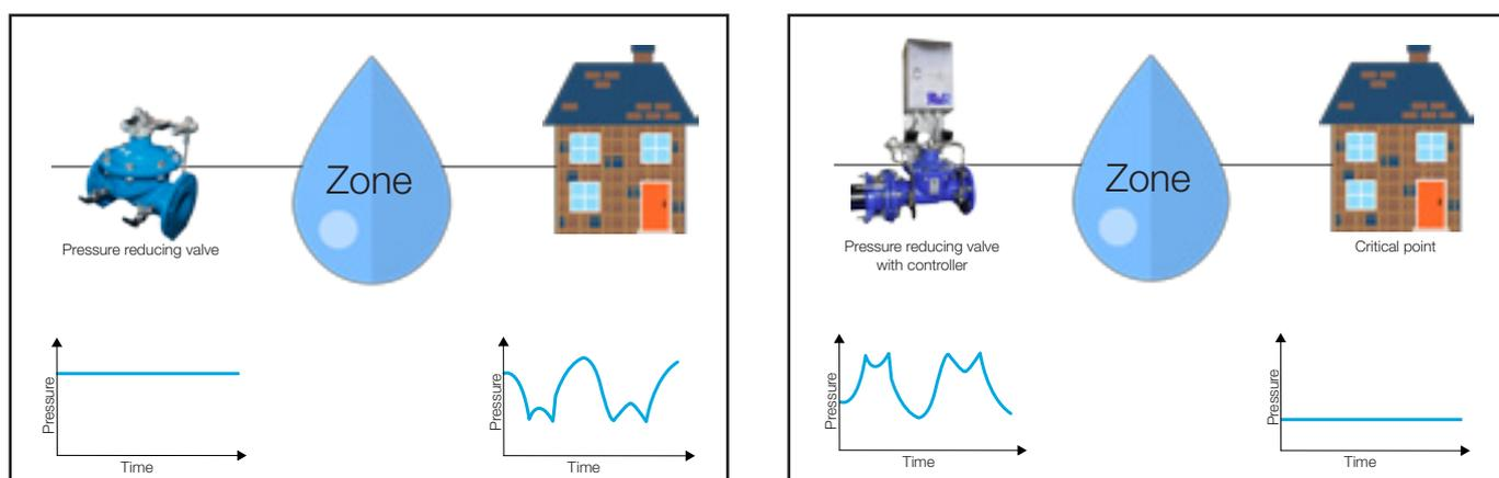
AVK offers various solutions to reduce water loss in the water distribution network. So far, we have primarily described leakage monitoring and leakage reduction by recommending high-quality and long-lasting shut-off gate valves. But another solution – which AVK is also able to be part of – is pressure management.
