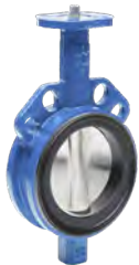
Series 820/00 Centric butterfly valve with loose liner Wafer Ductile iron DN25-1000 With any type of actuation
