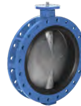
Series 820/20 Centric butterfly valve with loose liner U-section Ductile iron DN150-1600 With any type of actuation
