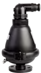
Series 701/75 Combination air valve Orifice sizes: Automatic: 12 mm 2 Kinetic: 804 mm 2 Reinforced nylon Inlet flange or 2" BSP thread PN 10 DN50-100
