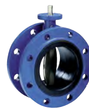
Series 75/20 Centric butterfly valve with fixed liner Double flanged short Ductile iron DN50-2000 With any type of actuation
