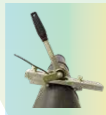
EXTERNAL DEBEADERS To remove external beads after butt fusion 63-125mm 90-400mm 355-630mm 400-900mm 710-1200mm
