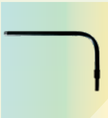
PE - STEEL CURVED TRANSITION PIECE (THREADED END) PE100 SDR11 Water PN16 Gas upon request d25x3/4" - 63x2"
