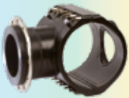
FLANGED BRANCH SADDLE UNDERCLAMP - FASTCUT PE100 Water PN16 Gas 10 Bar d250xDN150-630xDN150 Only available through approved fastcut installers
