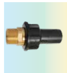
TRANSITION ADAPTOR BRASS DZR - MALE PE100 SDR11 Water PN16 Gas 10 Bar d20x1/2" - 125x4"
