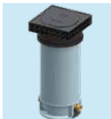
AVK PENTOBX WATER METER BOUNDARY BOX, CONTAMINATED GROUND GRADE B VERSION, SEALED SERIES 8054/5211 PN16 Polypropylene frame 3/4" BSP
